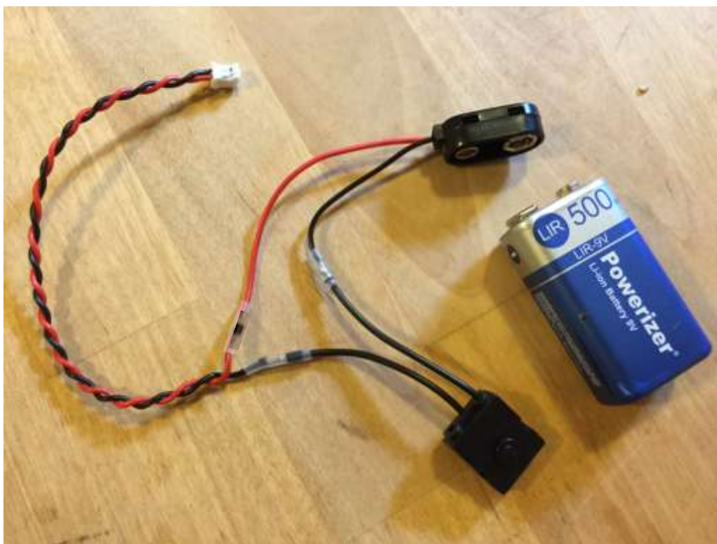
Power Supply Circuit with 9 Volt Lithium Rechargeable Battery
